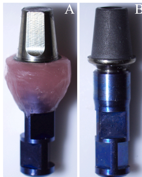
Fig. 2. Pretreatment of the standard abutment (A: Isolation of the margins; B: After sandblasting).
